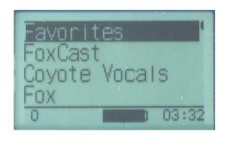
screen with the "Scroll Up" and "Scroll Down" buttons. As you scroll, the black highlight bar moves up and down, respectively. To select a menu item, push the "Select" button. To move back to the previous screen after making a selection, use the "Back/Menu" button.
